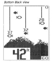
The 300TX remembers the Bottom Black setting when powered off.
